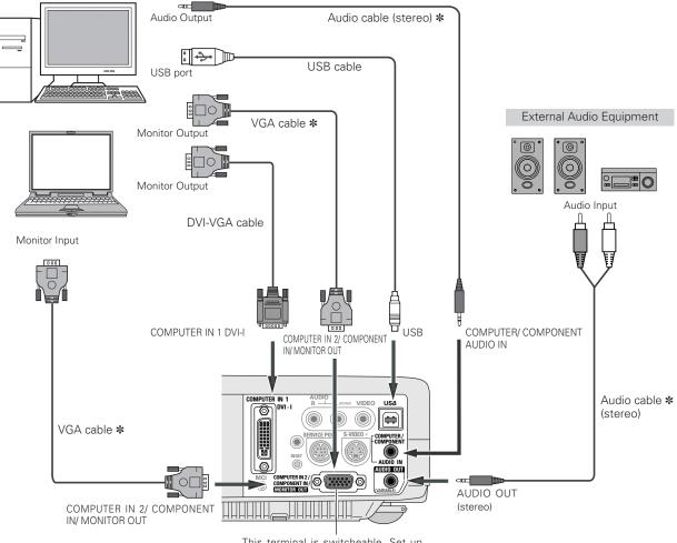
This terminal is switcheable. Set up the terminal as either Computer input or Monitor output. (See Page 44.)
