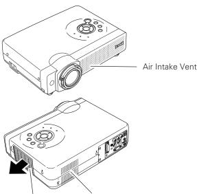
Exhaust Vent (Hot air exhaust)
