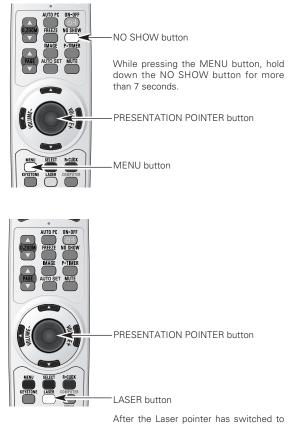
After the Laser pointer has switched to the Pointer, use the LASER button as the Pointer function ON-OFF switch. Press the LASER button toward the projector and see if it lights green.
